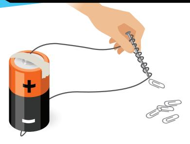
Electricity can help you make a magnet. When you send electricity through a piece of metal, it becomes magnetized. We call it an electromagnet. Electromagnets can be very, very strong. They are often used in manufacturing and to help lift heavy loads.
